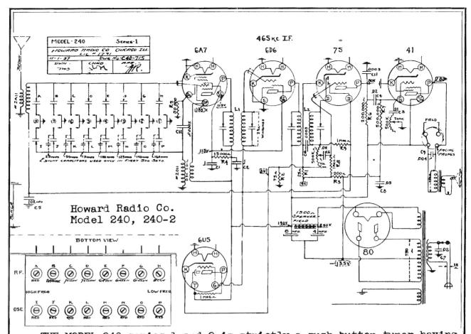
THE MODEL 240 series 1 and 2 is strictly a push-button tuner having no gang condenser. The eight push-button station selectors complete the ground circuit of the oscillator and R. F. tuned condensers previously set to whatever frequency desired. The eight circuits cover the complete range of the broadcast band from 540 to 1750 KC. The instructions for the set-up are shown.
