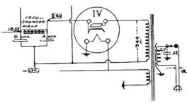
These sets can be easily aligned. The I.F. is set in the regular way. Then one station is tuned-in at a time and adjusted for maximum response. No other adjustments are needed.
