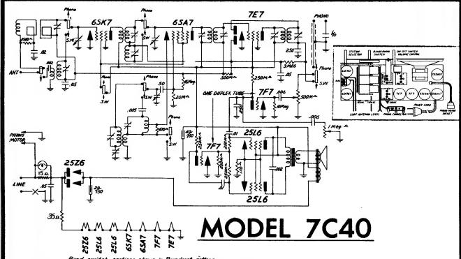
Band switch sections shown in Broadcast setting.
