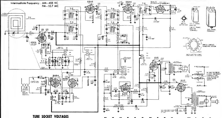
Socket voltages are shown on the schematic diagram at the tube socket terminals. All voltages are between the socket terminal and chassis ground. Plate, screen and cathode voltages were taken with a 1000 ohm-per-volt meter with a 300 volt scale used for plate and screen voltages. Audio grid voltages were read with a vacuum tube volt-meter. Conditions of measurement are:
