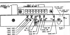
ELECTRICAL ADJUSTMENT—To align the set make the following preliminary adjustments: Set the tone pushbutton for treble tone; set the volume control at maximum; cennect the ground post of the signal generator to the radio chassis; connect the output meter across a 3.2-ohm output load; and allow the receiver and signal generator to warm up for several minutes.
