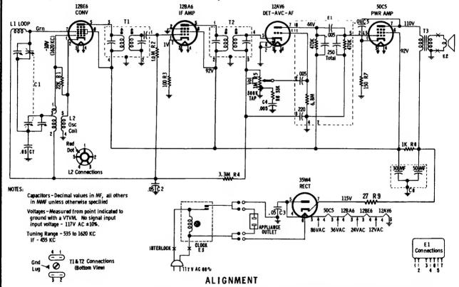
Use an isolation transformer between the power line and the receiver. If not available, connect low side of generator ground (outer chassis edges) through a . 1 mf capacitor. Connect a low range output meter across speaker voice coil and set volume control to maximum. Attenuate generator output to maintain . 40 volts on output meter to prevent overloading.
