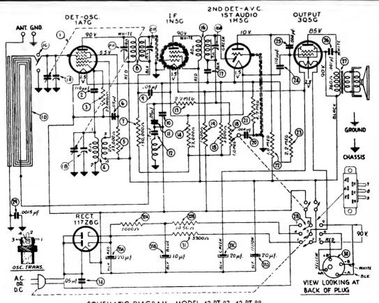
SCHEMATIC DIAGRAM—MODEL 42-PT-87, 42-PT-88 SOCKET VOLTAGES INDICATED ON THE DIAGRAM WERE MEASURED WITH A 1000 OHM PER VOLTMETER,
