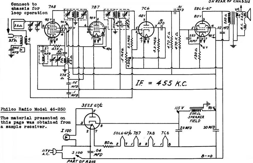
Voltage measurements made with a 20,000 ohms/volt meter.
