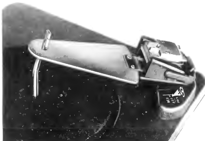
FIGURE 7. SPECIAL RECORD-SHELF GAUGE, SHOWN IN CORRECT POSITION
