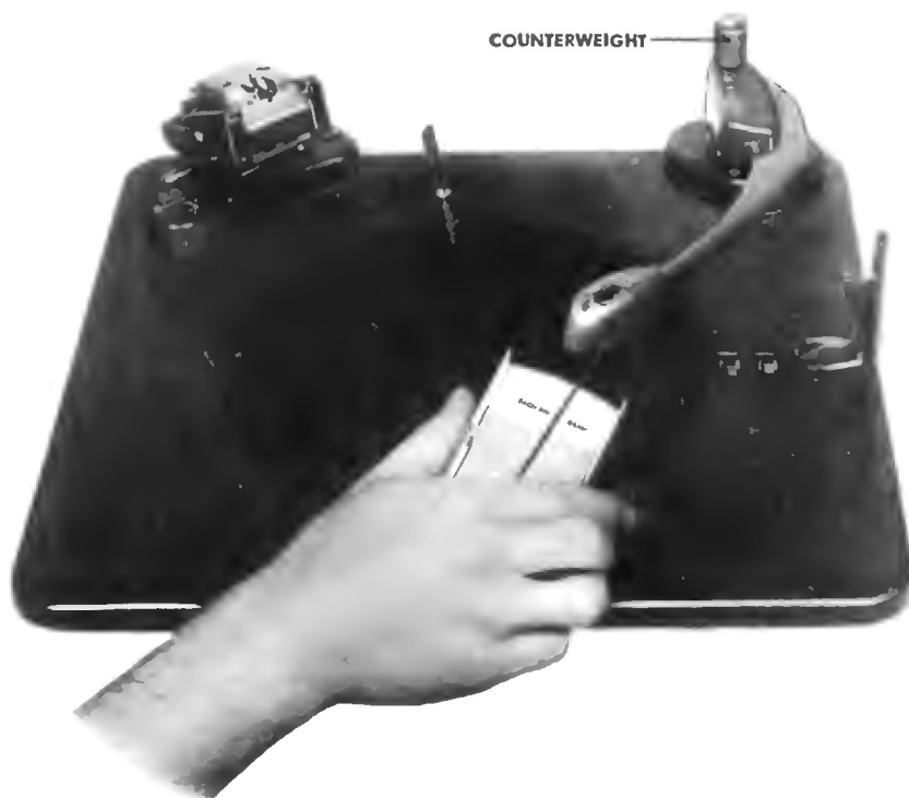
FIGURE 10. MEASURING HORIZONTAL FRICTION
