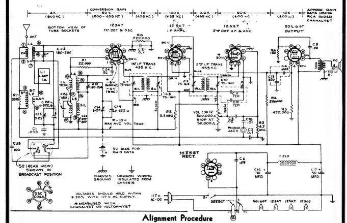
Output Meter Alignment.—If this method is used connect the meter across the voice coil and turn the receiver volume control to maximum.
