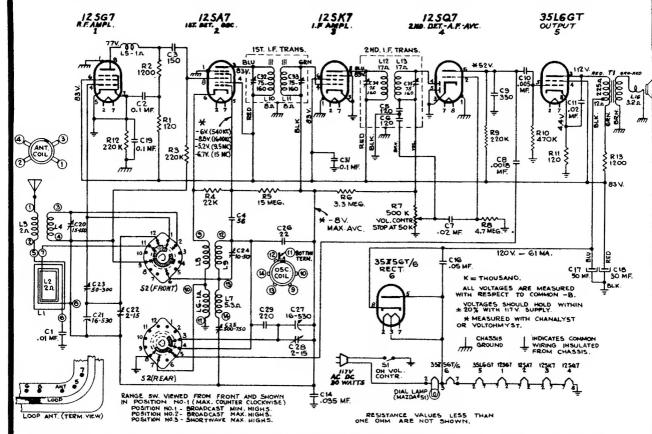
On some models, electrolytic capacitor (C17, C18) may be 20 Mfd./30 Mfd. The AVC bypass capacitor, (C14) may be .030 Mf.
