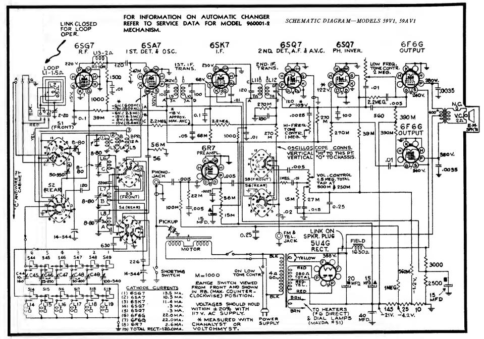
Cathode-Ray Alignment is the preferable method. Connections for the oscillograph are shown in the schematic diagram.
