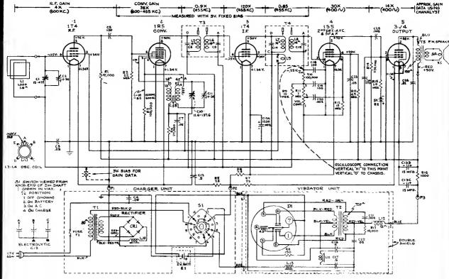
Cathode Ray Alignment is the preferable method. Connections for the oscilloscope are shown on the schematic diagram.
