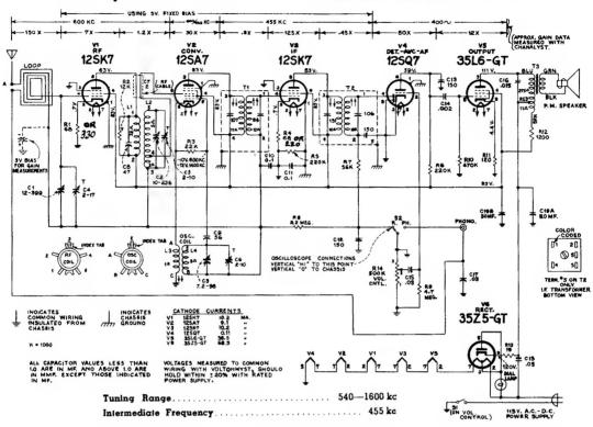
In some chassis an alternate filter capacitor is used which has three sections. The low voltage section (20 mf. 25 volts) is not used. The alternate capacitor is mounted on top of the chassis and is available as Stock No. 73975.
