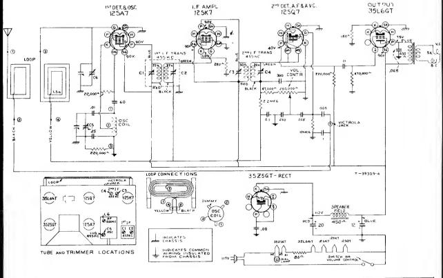
Output Meter Alignment.—Connect the meter across the voice coil, and turn the receiver volume control to maximum.
