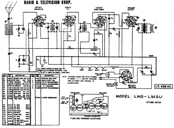
Voltages shown on the circuit diagram are from socket terminals to ground buss. In measuring voltages use a voltmeter having a resistance of at least 1000 ohms per volt. Allowances should be made for variations in line voltage.
