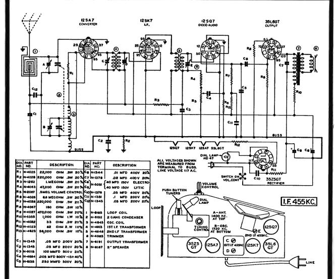
GENERAL DATA. The alignment of this receiver requires the use of a test oscillator that will cover the frequencies of 455, 600, 1400 and 1720 KC and an output meter to be connected across the primary or secondary of the output transformer. If possible, all alignments should be made with the volume control on maximum and the test ascillator output as low as possible to prevent the AVC from operating and giving false readings
