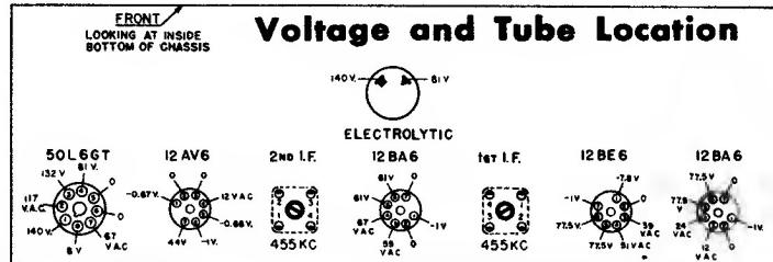
Measurements are made at 117V line, using electronic Voltmeter. Except where otherwise indicated, voltages are D.C. and are positive with respect to the reference point which is the common Black-White lead.
