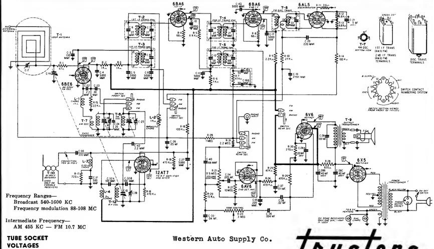
Socket voltages are shown on the schematic diagram at the tube socket terminals. All voltages are between the socket terminal and chassis ground. Plate, screen and cathode voltages were taken with a 1000 ohm-per-volt meter with a 300 volt scale used for plate and screen voltages. Audio grid voltages were read with a vacuum tube volt-meter. Conditions of measurement are:
