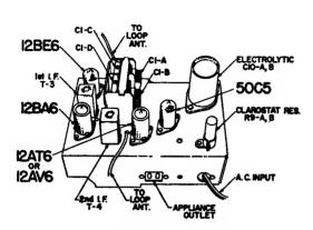
NOTE: Resistor R9A-B may be of either the Muter or Clarostat type as illustrated.
