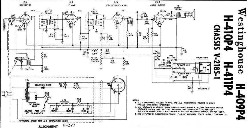
Signal Connect Signal Generator Radio Step Generator to -Frequency Dial Adjust for Maximum Output -1 Stator of RF section of tuning 455 kc. Minimum Top and bottom slugs of 2nd and 1st IF transcapacitor C1 through a .01 mfd formers in order given, SEE NOTE, capacity capacitor 2 Radiated signal 1625 kc. 1625 kc. Osc. trimmer "D" (rock-in) Ant. trimmer "B" 3 1400 kc. Radiated signal 1400 kc. Repeat steps 2 and 3
