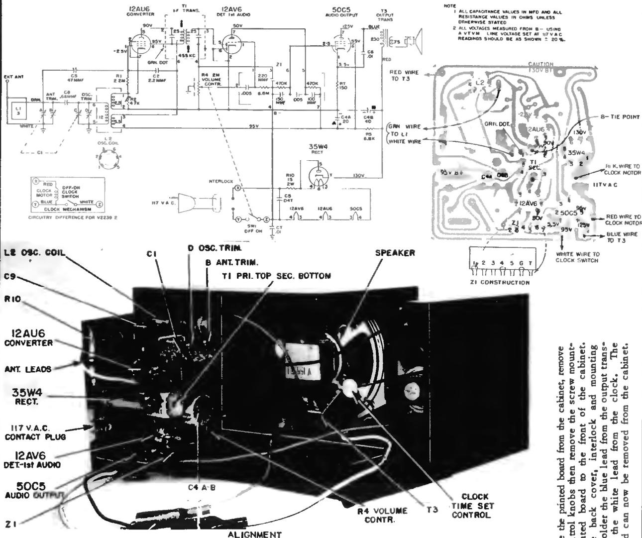
It is recommended that the chassis be isolated from the power line by means of an isolation transformer. While making the following adjustments, keep the volume control set for maximum output and the signal generator output attenuated as much as possible. Connect VTVM across voice coil.
