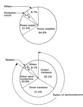
Fig. 58 Pie charts for faulty blocks and components
