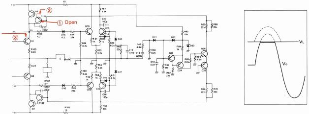
Fig. 23 Vo is clipped when Q101 opens
