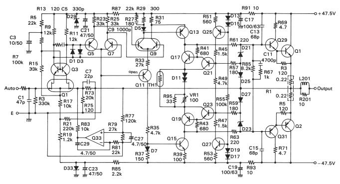
Fig. 93 Suspected components of "No sound although Protection Relay turns on."
