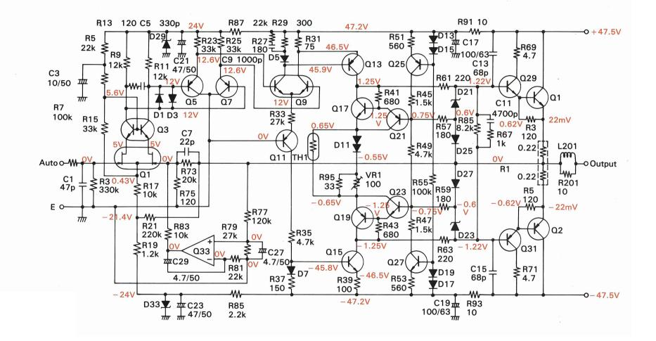
Fig. 72 Voltages under normal condition (with no input)
