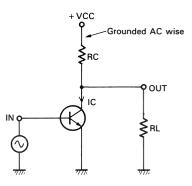
Fig. 40 Emitter-grounded amplifier
