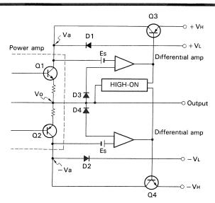
Fig. 6 Simplified circuit of DPS system
