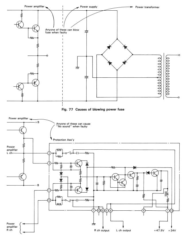
Fig. 78 Causes of no sound
