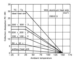
Fig. 60 Ambient temperature versus allowable collector dissipation (Pc)
