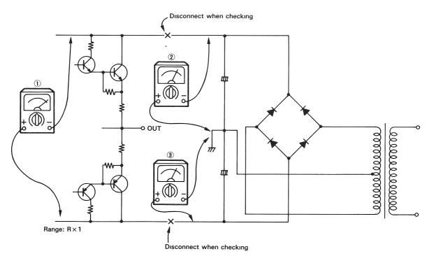
Fig. 79 Finding faulty block - Primary fuse blows out.
