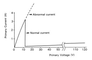
Fig. 82-c Primary voltage vs primary current
