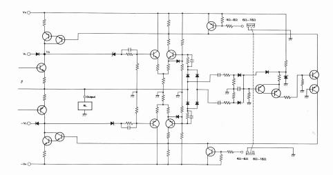
Fig. 24 A-70 Dynamic power supply circuit
