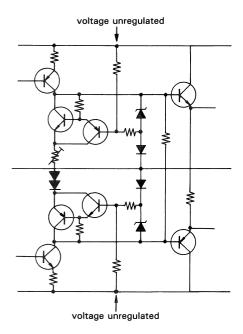
Fig. 26 Fed from voltage-unregulated power source
