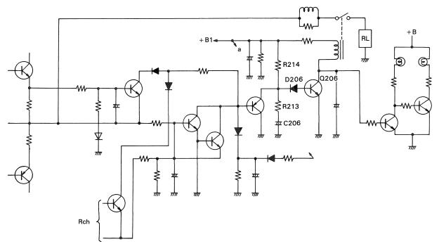
Fig. 100 Protection circuit
