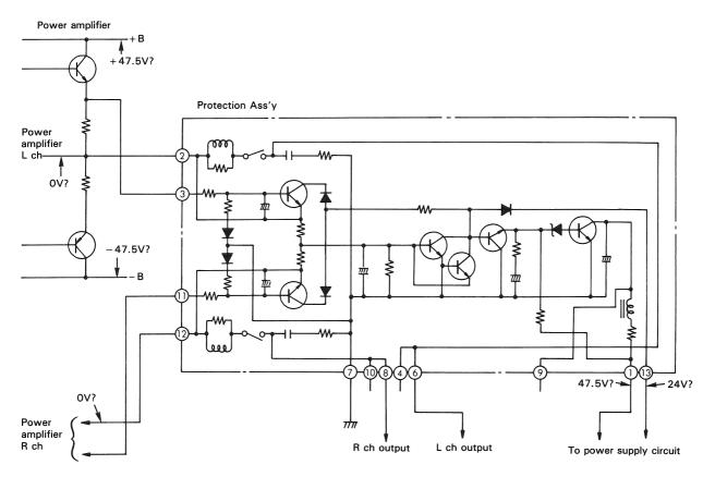
Fig. 80 Finding faulty block - No sound
