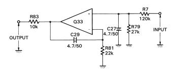
Fig. 30 DC servo circuit
