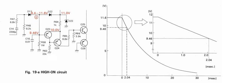
D22 bypasses the current and avoids excessive reverse voltage and protects Q23. D23 keeps Q23's VE constant. In A-80, it is held at 11 V.
