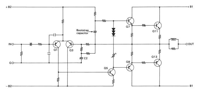
Fig. 8 All-Stage Direct-Coupled SEPP Amplifier
