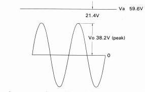
Fig. 11-b Output and power supply waveforms when speakers are disconnected
