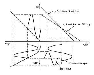
Fig. 42 Characteristics with ordinary resistor load
