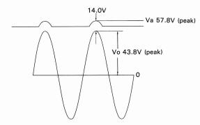
Fig. 13-b Output and power supply voltage waveforms
