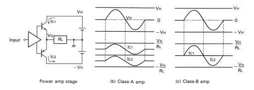
Fig. 3 Voltage (current) waveforms of class-A and class-B amplifiers
