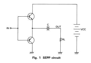
Note: Single-Ended Push-Pull (SEPP) circuit SEPP circuit is a push-pull circuit in which two transistors are connected serially DC-wise and in parallel AC-wise and the output of the positive half cycle and that of the negative half cycle are taken out of a common point. Being parallel ACwise, the output impedance can be made low. Having low internal impedance, it can drive speakers directly. And it is being employed in most power amplifiers.
