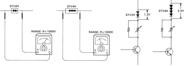
Fig. 74 Checking varistor (1)
