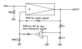
Fig. 29 Basic operation of amplifier with DC servo circuit
