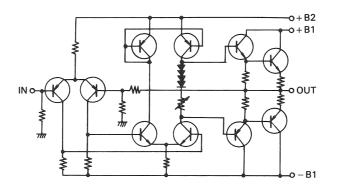
Fig. 4 All-Stage Direct-Coupled SEPP DC Amplifier
