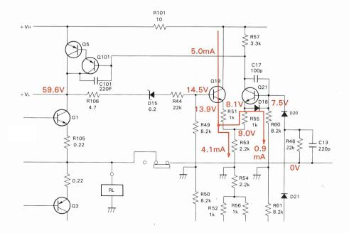
Fig. 9 Voltage and current values at each point
