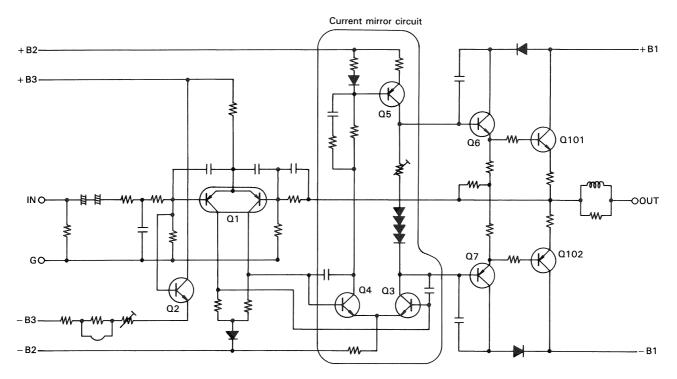
Fig. 10 All-Stage Direct-Coupled SEPP DC Amplifier
