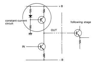
Fig. 44 Amplifying circuit with constant-current load
