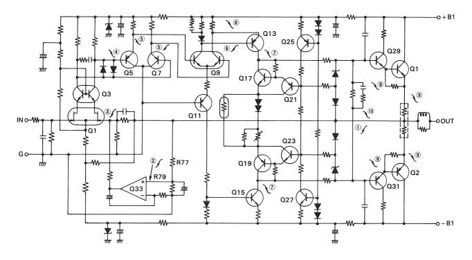
Fig. 34 Operation of DC servo circuit
