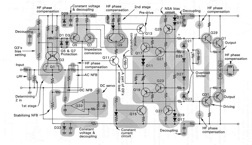
Fig. 28 Role of each part in A-7 power amplifier
