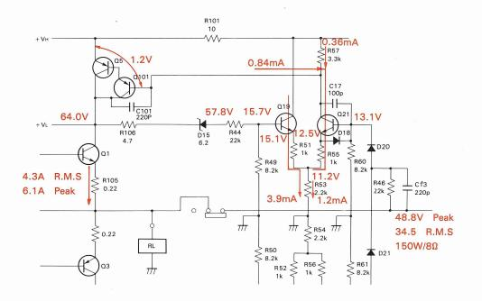
Fig. 12-a Voltage and current reading when producing 150W signals
