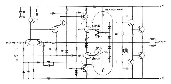
Fig. 11 Non-Switching Amplifier
