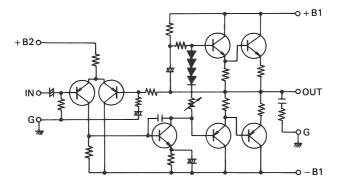
Fig. 3 All-Stage Direct-Coupled SEPP Amplifier
