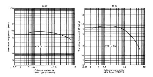
Fig. 56 f<sub>T</sub>-I<sub>C</sub> characteristics
