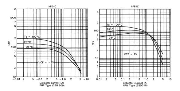
Fig. 55 h<sub>FE</sub>-I<sub>C</sub> characteristic
