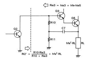
Fig. 48 Load of Q<sub>2</sub> with bootstrap circuit
