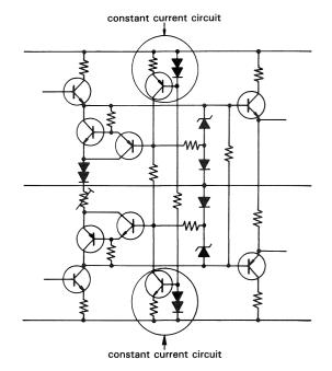
Fig. 25 Fed from constant-current power source
