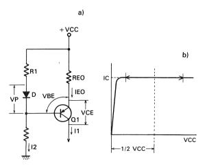
Fig. 41 V<sub>CC</sub> - I<sub>C</sub> Constant-current circuit and characteristic
