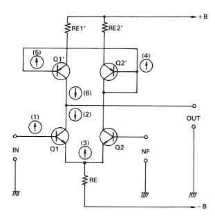
Fig. 51 Current mirror circuit in the input stage
