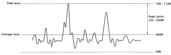
Fig. 1 Audio signal level
