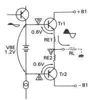
Fig. 20 Biasing of class-B Amplifier
