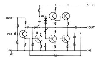
Fig. 2 Standard Single-Ended Push-Pull Amplifier
