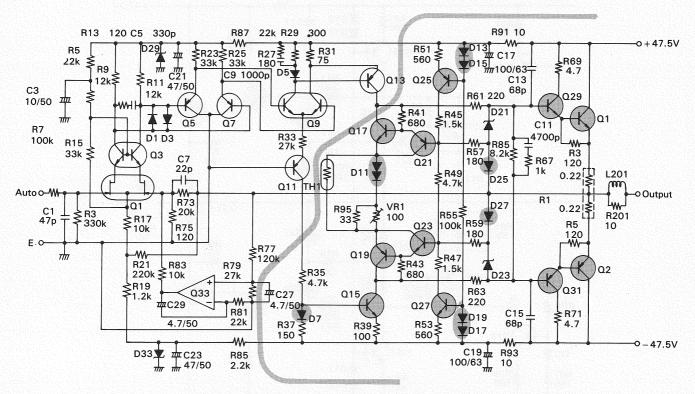
Fig. 85 Suspected components when fuse blows
