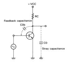
Fig. 38 Existence of equivalent capacitance
