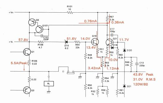
Fig. 13-a Voltage and current readings when output is 120W signal
