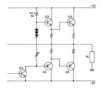
Fig. 45 Power Amplifier without bootstrap circuit
