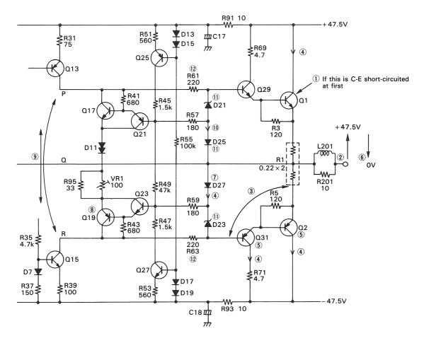
Fig. 71 Process of damage
