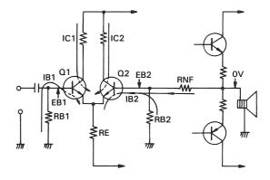
Fig. 52 1st-stage of All-stage Direct-coupled DC Amplifier
