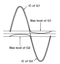
Fig. 24 Waveform of collector currents
