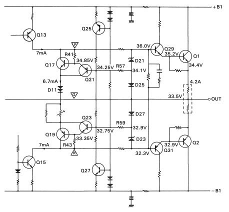
Fig. 23 Momentary potential at positive peak, 70W output
