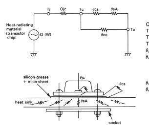
Fig. 62 Thermal resistance in the radiating route
