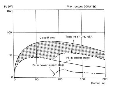
Fig. 5 Output power VS. dissipation
