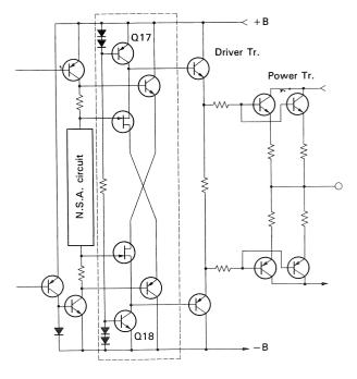
Fig. 33 Buffer circuits in A-90
