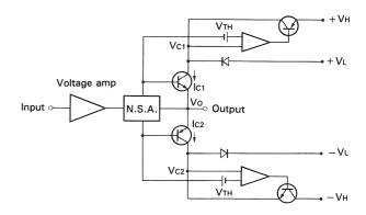
Fig. 2 Simplified diagram of DPS system
