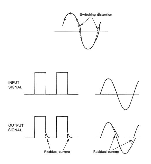
Fig. 19 Generation of switching distortion
