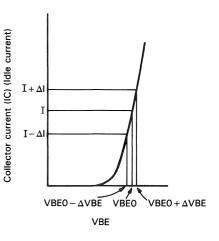
Fig. 17 Elimination of crossover distortion by flowing idle current
