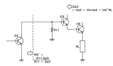
Fig. 47 Load of  $Q_2$  without bootstrap circuit
