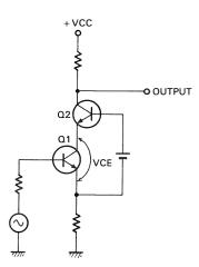
Fig. 39  $V_{CE}$  setting of cascode amplifier
