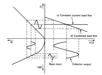
Fig. 43 Characteristics with constant-current load
