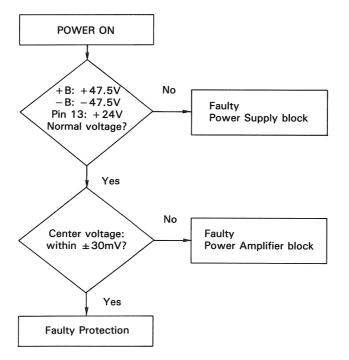
Fig. 81 Finding faulty block
