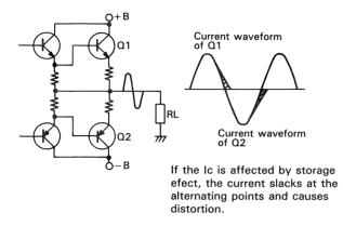
Fig. 63 Wave deformed by storage effect of electron
