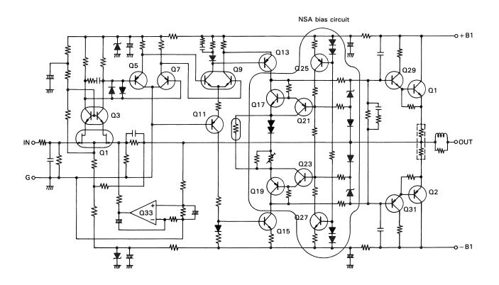
Fig. 12 Non-Switching Amplifier (with DC servo circuit)
