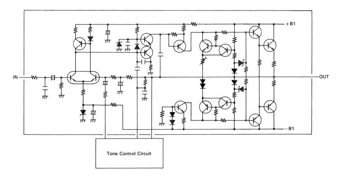
Fig. 5 Non-Switching Amplifier
