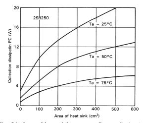
Fig. 61 Area of heat sink versus collector dissipation
