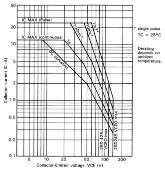
Fig. 64 ASO characteristic of power transistor
