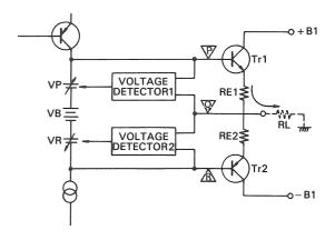
Fig. 21 Biasing of Non-Switching Amplifier
