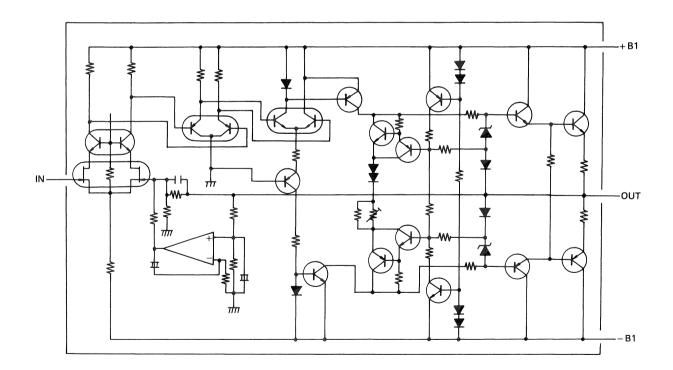
Fig. 6 Non-Switching Amplifier (with DC servo circuit)
