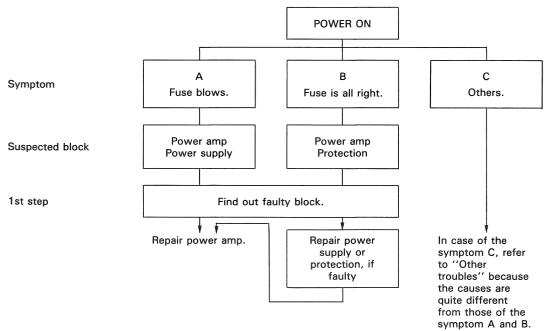
Fig. 76 Confirmation of defect
