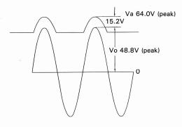
Fig. 12-b Output and power supply voltage waveforms
