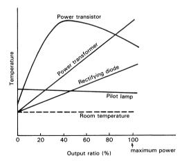
Fig. 59 Output ratio versus temperature rise
