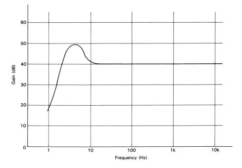
Fig. 9 Frequency response of standard SEPP amplifier
