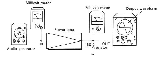
Fig. 87 Final check after repairing
