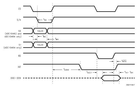
FIGURE 1. Mode 1. The conversion time  $(t_{\mbox{\scriptsize CONV}})$  is set by the internal timer.
