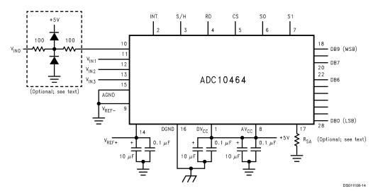
FIGURE 4. Typical Connection. Note the multiple bypass capacitors on the reference and power supply pins. If  $V_{REF-}$  is not grounded, it should also be bypassed to analog ground using multiple capacitors (see 5.0 "Power Supply Considerations"). AGND and DGND should be at the same potential.  $V_{INO}$  is shown with an input protection network. Pin 17 is normally left open, but optional "speedup" resistor  $R_{SA}$  can be used to reduce the conversion time.
