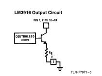
Outputs may be run in saturation with no adverse effects, making it possible to directly drive logic. The effective saturation resistance of the output transistors, equal to R<sub>E</sub> plus the transistors' collector resistance, is about 50 $\Omega$ . It's also possible to drive LEDs from rectified AC with no filtering. To avoid oscillations, the LED supply should be bypassed with a 2.2  $\mu$ F tantalum or 10  $\mu$ F aluminum electrolytic capacitor.
