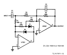
FIGURE 5. Precision Full-Wave Average Detector
