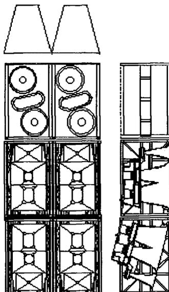
**Figure 2.** HLA array for medium size venue (curved front)
