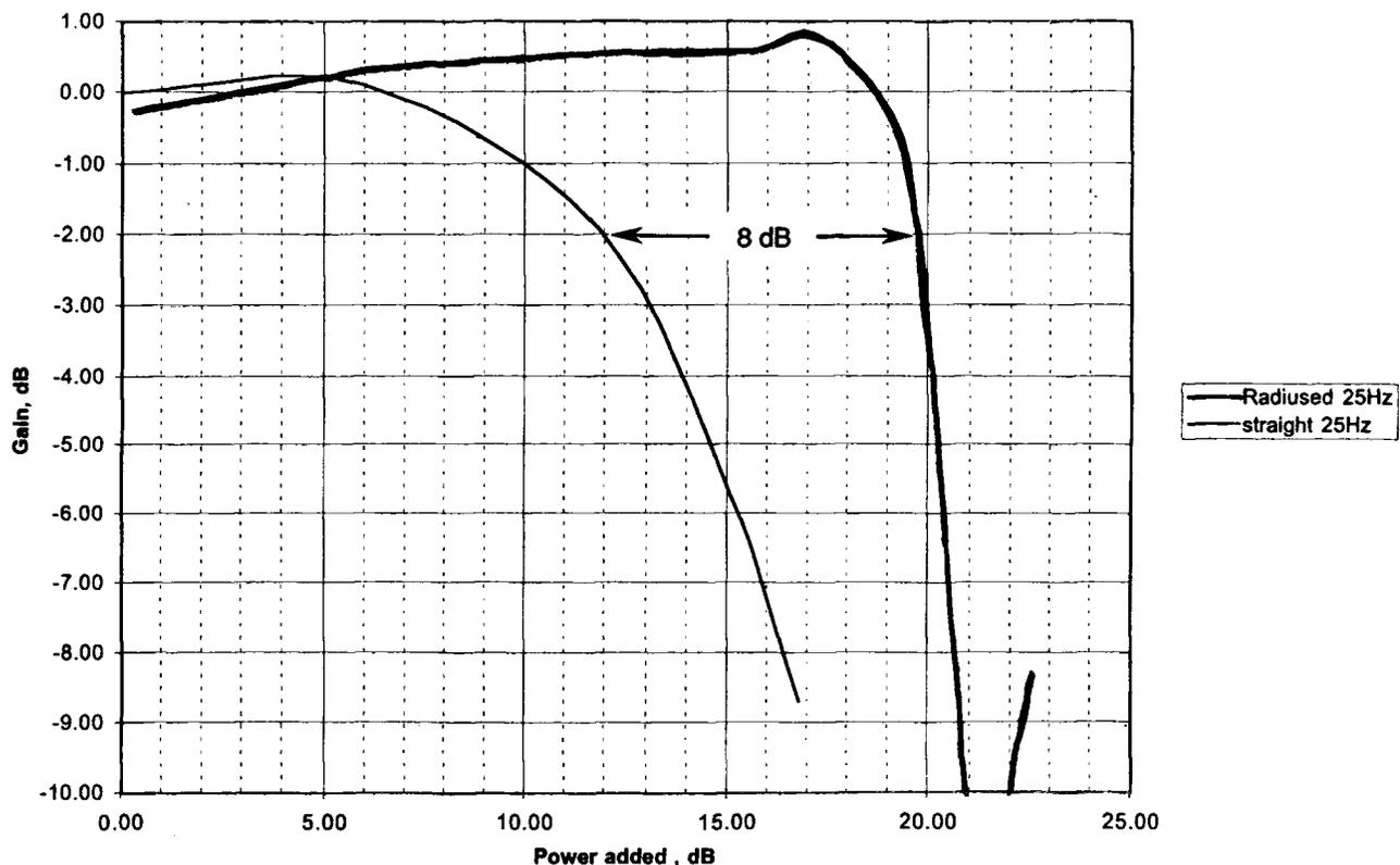
improvement in output level over standard porting at the point where both porting systems exhibit 2 dB of compression.
