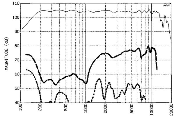
Finally, we want to point out the extremely flat on-axis response of the 4895 system. This illustrates the inherent linearity and smooth response of the MultiBand Waveguide, augmented by the capability of the JBL DSC 280 controller in fine-tuning and time aligning of complex systems.
