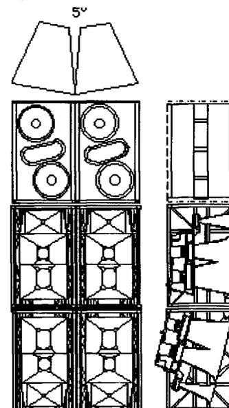
be tilted 15° as a unit while the SpaceFrame remains fixed. For wider coverage the two vertical stacks may be splayed outward as shown in Figure 2. The goal is to use a minimum number of high intensity, highly directive sources so that each listener hears a minimum number of effective sources, with a resultant high direct-to-reverberant ratio.
