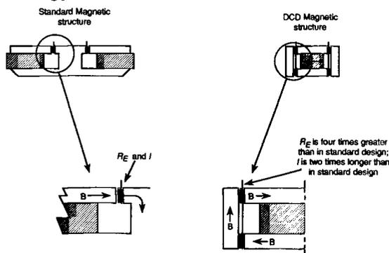
coil has an electrical resistance,  $R_E$ . These quantities establish the value of  $(Bl)^2/R_E$ .
