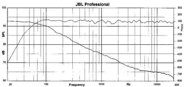
The phase curve shows a progressively larger negative shift with respect to frequency. For this system, the group delay ( $-df/dw$ ) would then tend to be constant over most of the frequency range, since the phase response is of constant slope over most of the range.
