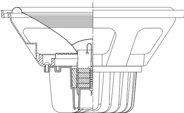
We can get a clearer understanding of the advantages of Differential Drive by comparing it with an equivalent single coil structure, as shown in Figure 2. We use the term “equivalent” in that this comparison of both motor structures will have the same electromechanical coupling coefficient,  $(BI)^2/R_e$ , and also the same moving mass. We will analyze the two structures in parallel, so to speak, in order to
