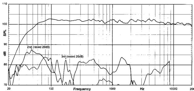
Note in Figure 10A that the level of both distortion components in the frequency range above 100 Hz is -40 dB or lower, relative to the fundamental. This corresponds to distortion of less than 1% and represents unusually fine performance at such a high acoustical output level. The data taken at 102 dB shows distortion components above 100 Hz lying - 35 dB or lower, corresponding to distortion in the range of 2% — again, remarkably fine performance.
