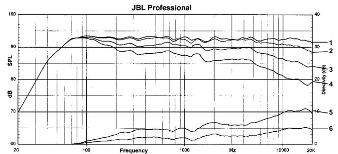
As an example of an earlier three-way loudspeaker system designed with attention primarily on attaining a flat on-axis response, we show the data of Figure 9. Note that the on-axis curve is fairly flat, but that the listening window and early reflections curves show clear irregularities.
