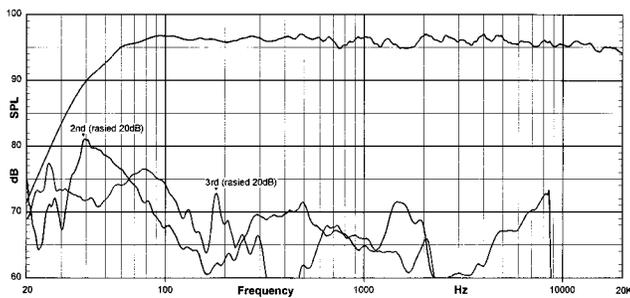
**Figure 10B. 102dB Distortion Graph**
