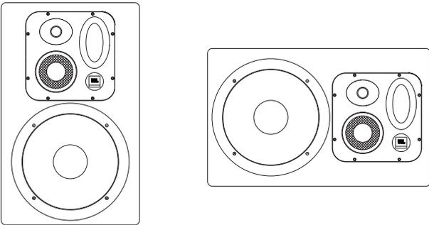
The baffle itself is made of a carbon fiber composite that has a thickness of 38 mm. It is virtually resonance free and is complemented by enclosure walls that are braced. As we engineer better transducers with lower distortion, we find that enclosure resonances, even those produced by conventionally good, sturdy design, may be heard as such and contribute to a distortion “signature”. It is the next step in refinement of system performance to reduce them.
