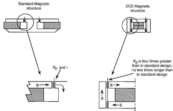
Now, let us look at the Differential Drive topology shown at 2B. In this design there are two magnetic gaps with opposite flux. The two voice coils are connected in reverse so that the mechanical forces they produce will add (be in-phase). For the moving mass to remain the same, the two voice coils must have the same height and half the thickness as in the standard case. The value of  $B$  will remain the same.
