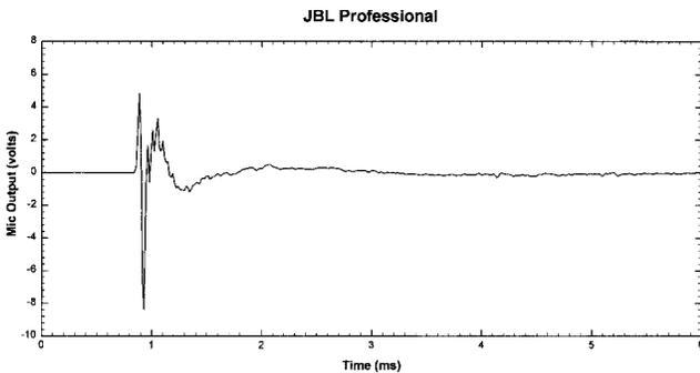
Figure 14 shows the impulse response of the LSR32 System. Note the smooth and rapid decay of the impulse response.
